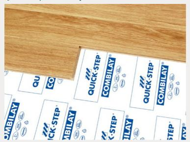
Combi-Lay Standard is a good quality, medium density polyolefin underlay for all floating floor applications. It incorporates a continuous clear damp-proof with 100mm overlap and integrated "peel and stick". The inclusion of a continuous damp proof is a requirement under most floating floor installations. With Combi-Lay, the need for additional damp proof layers is almost always avoided\*, making installations quicker and more cost effective.
