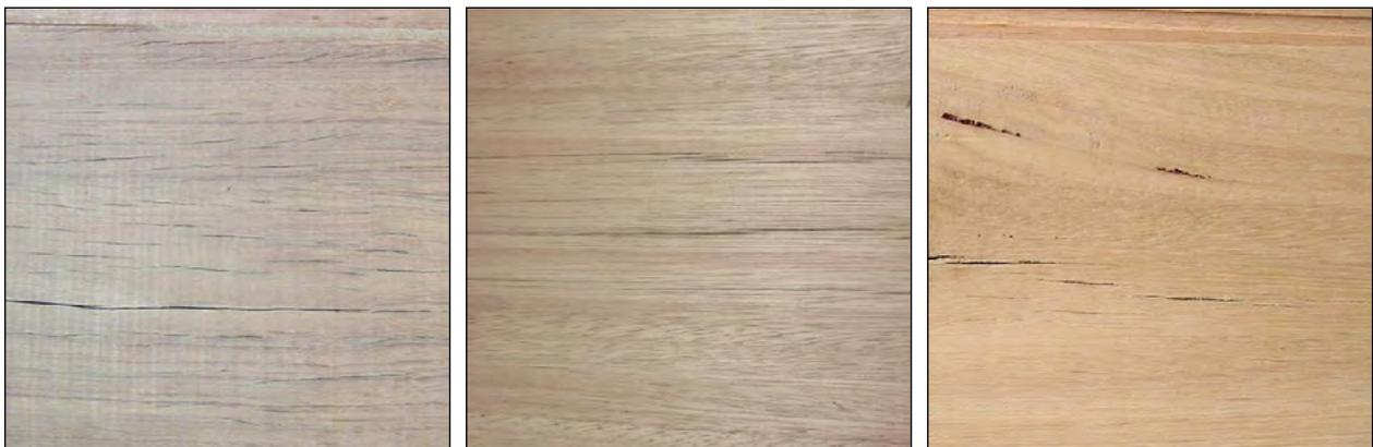
Checks are a separation of the wood fibre and differ from a split in that they do not travel from one surface of a board to another. They can often occur with rapid drying and be over much of the board surface. However, grain
