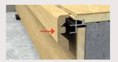
6. Press the Incizo® profile onto the sub-profile.
